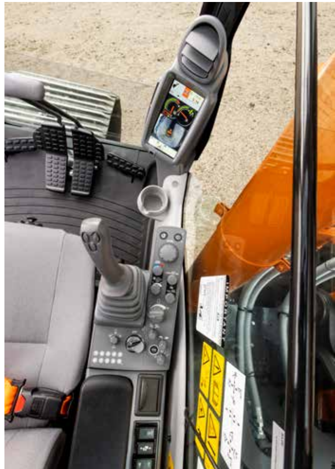
Comfortable cab space. ROPS certified CRESV cab.
