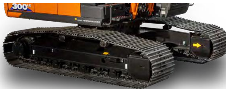
Reinforced undercarriage and increased crossbeam size and strength increase durability.
