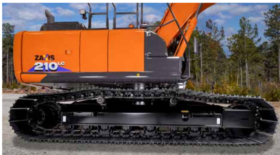
Reinforced undercarriage and increased crossbeam size and strength increase durability.
