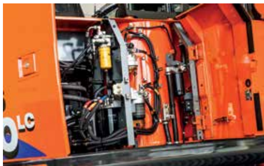
A larger electric fuel pump and enhanced injection system provide a precise quantity of pressurized fuel used to achieve more-efficient engine performance and reduce fuel consumption.
