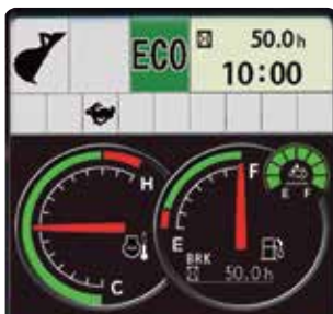
Checking DEF fluid level through Multi-function monitor.
