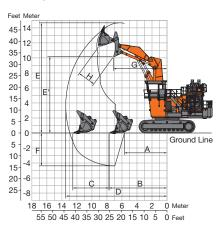
Bucket Capacity ISO 7456 Heaped 2:1 12.0 m<sup>3</sup> (15.7 cu. yd.) 5 660 mm (18 ft. 7 in.)
