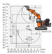
BE-arm length Bucket capacity ISO 7451: 2007 Maximum Digging Reach
