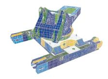
Computer assisted analysis has been Improved Hitachi track link design used to determine the most effective mitigates premature failure of the master design for frame longevity, to ensure the pin, increasing durability. machine withstands the demands of any mining operation.
