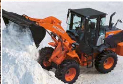
Torque proportioning differentials reduce tire slippage in wet or wintry conditions.
