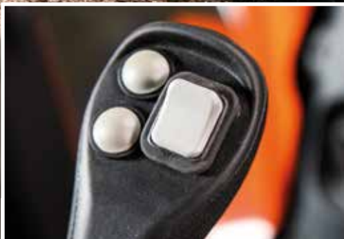
The quick power switch increases power when required.
