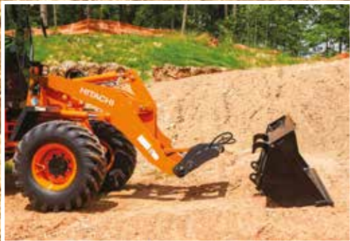
Universal Quick Couple allows seamless transition (ZW80-5b).
