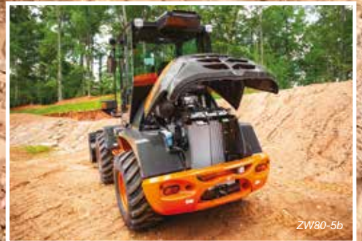
Easy access for maintenance from ground level.
