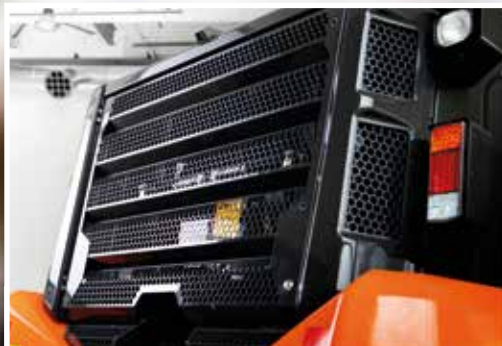
New rear grill protects radiator compartment.
