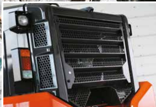
New rear grill protects radiator compartment.
