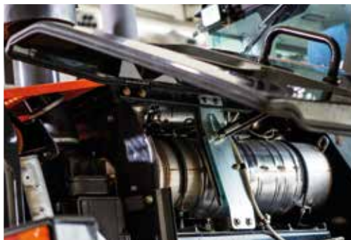
NO DPF SCR system reduces emissions.
