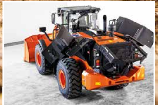
Easy access for maintenance from ground level.
