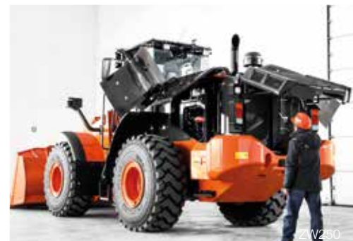
Easy access to the engine compartment.
