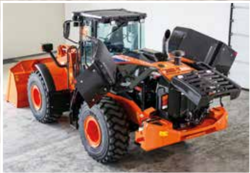
Ground level access for easy maintenance.
