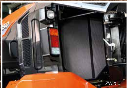
Optional clog resistant cooling cores enhance durability.
